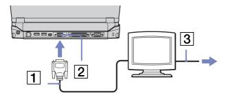
If the main unit is docked, you can only use the monitor connector on the docking station.
